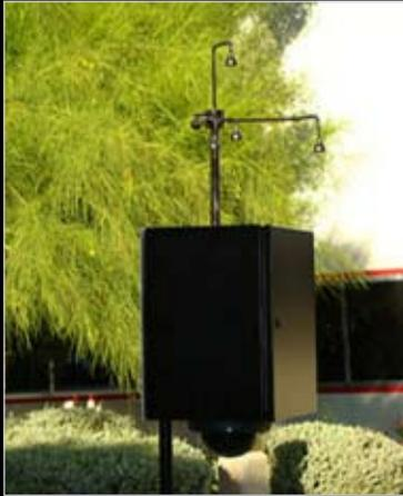
The system is a breakthrough technology that recognizes gunshots and explosions and sends range and bearing details to cameras which can then locate the source of the event.
